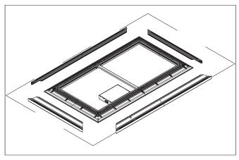
**6b.** Slide the long Velvet Cover onto the border of the frame with the same length. Lift the corresponding border a tiny bit (1/4") off the ground and slide the Velvet Cover onto the border with its long side facing up as shown below.
