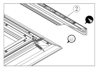
Make sure the Aluminum Velvet Cover you are trying to put on is marked the same number according to the Inner Frame.
