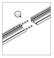
**2b.** (Optional) On select large sized screens only, you will be provided with a middle Support Bar. If you have a Support Bar, lay out the Support Bar as shown below.
