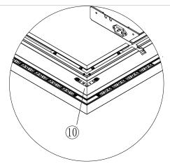
**7c.** Connect the LED Connectors to the two LED strips as shown below: Make sure the connectors and sockets are all the way in and all four pins are properly connected.
