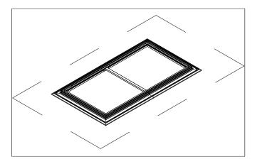
Make sure the corners are at 90 degree angles and that the horizontal frames are straight before proceeding. There should be no gap between the horizontal frames and less than 1mm gap in the four corners.
