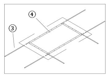
The four plastic rods of the same length make up the two horizontal sides, while the two rods of the same length make up the vertical side of the fabric.
