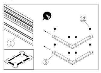
**1f.** The screen should now be as shown below. The Inner Frame pieces can now be joined together with the brackets from previous steps.
