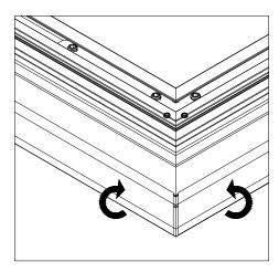
**5c.** The fabric and the frame will be joined with springs. First the corners will be secured, then the sides will be secured starting from the corners and moving towards the middle. The shorter sides should be secured first for optimal tension. The priority that the springs should be secured is below.
