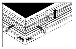
Repeat the above steps for other springs near the wrinkles. Repeat as necessary until there are no more wrinkles in the screen fabric. If necessary, you may also use your hands for this operation described above. Please wear protective gloves and only pull on the sleeve of the fabric.
