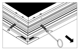
Pull the Installation Hook towards back of the frame. This will stretch and wrap the screen fabric around the frame.
