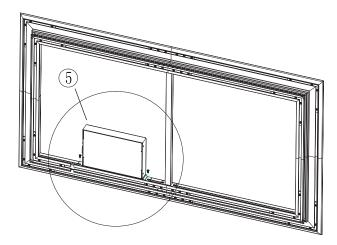
**3b.** Slide the anchors into the proper position. Insert the screws and mount the LED Control Box as shown below. Mount the box the furthest to the back of the frame as possible, align the screws, then tighten them.
