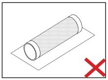
Do not lay the roller directly onto the ground for a long period of time
