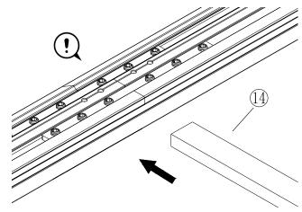
**2d.** Insert the Corner Brackets into the vertical frame and the horizontal frame. Align the corner and push the two frames towards the corner. Make sure there is no gap bigger than 1mm, then tighten the Set Screws. If you have a Support Bar, see 2e.
