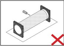
Avoid using sharp objects around the screen material and roller.
