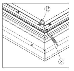
**5e.** Use the installation hook provided to mount the springs. Latch the shorter hook onto the lip of the frame. Carefully pull the larger hook through the hole in the screen and around the plastic rod. Make sure that the spring is only around the rod and not caught on any fabric before you release it.
