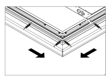
Pull on the fabric and wrap the fabric around the corner until the corner is flat and free of wrinkles. You may use your hands for this operation. Please wear protective gloves and only pull on the sleeve of the fabric.
