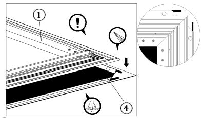
Do not stand the frame on its corner as the sharp edge will damage the screen fabric.
