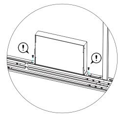
You want to position the LED Control Box that the cable coming out of the control box is able to go through the slot on the frame and reach the LED strips.
