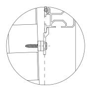
As illustrated above and below, use washers provided in the packaging underneath the Mounting Brackets or Mounting Plates to make the screen sitting upright when the wall is not completely flat.
