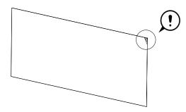
Repeat step 5g. Remove the springs around the corners and move the material towards the corner as shown below. Remount the springs and pull on the fabric manually as described above to get rid of wrinkles in the corner of the fabric.
