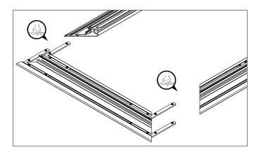
Make sure you align both sides properly and center the bracket inside its slot before tightening the Set Screws on either sides.
