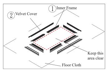
Do not leave any parts or tools within the dotted area indicated above during the whole assembly and installation process. Keep clear at all times.
