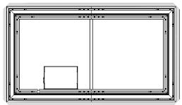
The black backing will go **between** the screen material and the frame. The smoother side of the black backing is the front, lay the front of the material towards the back of the screen fabric you put on the floor in step 4a.. Then put the frame on top of the black backing.
