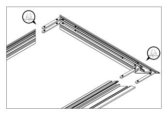
**2f.** After all the frame pieces are joined together, it will look similar to below. Check and tighten all Set Screws as they will not be able to accessible once the Outer Frame is installed.
