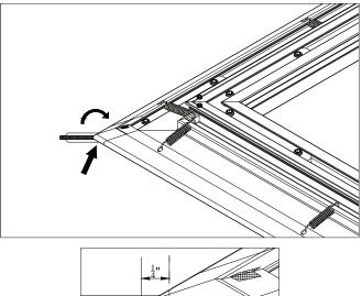
Flip the flap of material over and stick the Velcro towards the frame as shown below:
