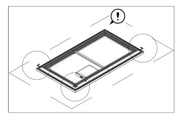
The corner furthest away from the LED Control Box is the corner that does not require a LED Connector.
