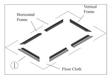
**1d.** Insert the two of Joint Brackets into the slots of the two horizontal frame pieces. Position the brackets so they are centered, insert the Set Screws, and do not tighten the set screws as shown below.
