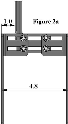
Forward adjustment when the Depth Support has clearance to move past 0
