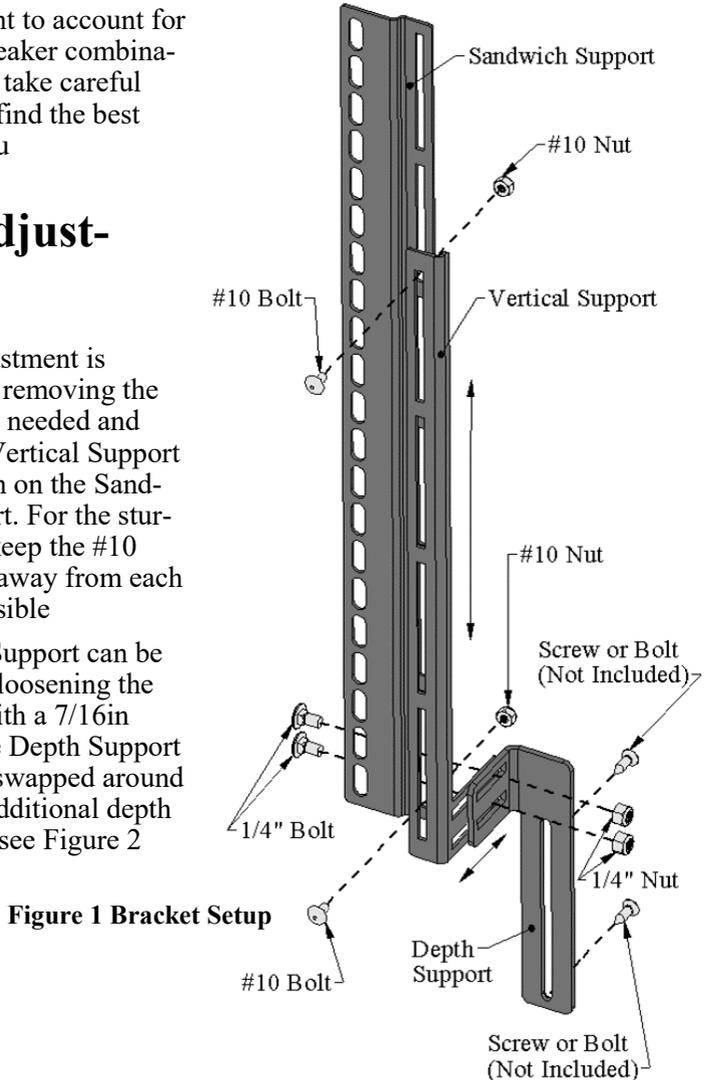
Figure 1 Bracket Setup
