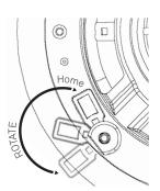
Insert the speaker into the hole and turn each screw clockwise. The toggle clamps will rotate outward to engage the ceiling material as shown. Before tightening the three screws, orient the speaker toward the listening area. Tighten all the screws. CAUTION: DO NOT OVER-TIGHTEN THE CLAMPS. Too much torque may damage the toggle, causing the speaker not to seat securely. A snug fit is all that is necessary to assure proper performance.
