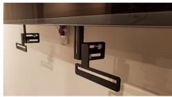
Secure the UM1-A adapter bracket to the back of the SONOS® ARC by using the provided hardware in this recommended order: 18mm M5 bolt, lock washer, flat washer, fender washer and then into the SONOS® ARC using the hex key. We **strongly suggest** two people perform this action to ensure that you do not drop the SONOS® ARC while securing to the UM1-A
