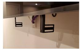
Replace with the UM1-A adapter bracket using the 1/4" carriage bolts and nylon nuts you removed
